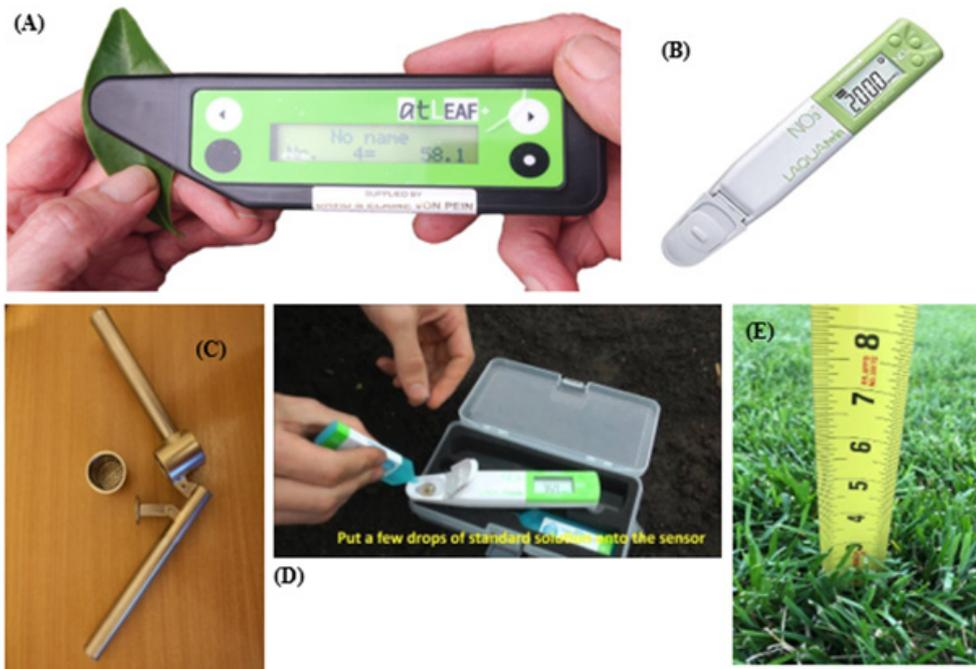
**Figure 2:** (A) Chlorophyll meter; (B) Nitrate meter; (C) Garlic Press/Sap Squeezer; (D) Nitrate meter calibration (E) Growth measurement using ruler.
