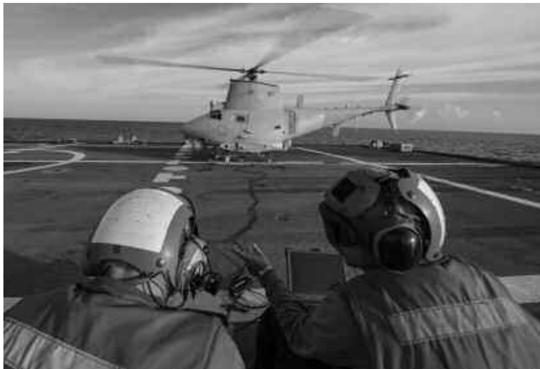
Sailors aboard the US Navy LCS Fort Worth (LCS-3) prepare to launch a MQ-8B Fire Scout UAV during an Asian deployment in 2015. Although seemingly offering manpower savings, UAVs still need to be flown and maintained. (US Navy)
