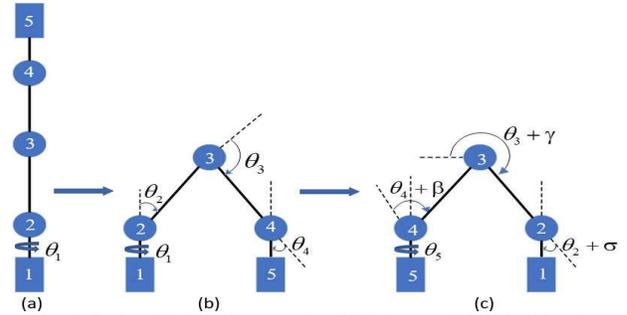
Fig. 1. Cycle-1 Walking Pattern of an E-Walker: (a) Initial Position (b) Phase-1 and (c) Phase-2
