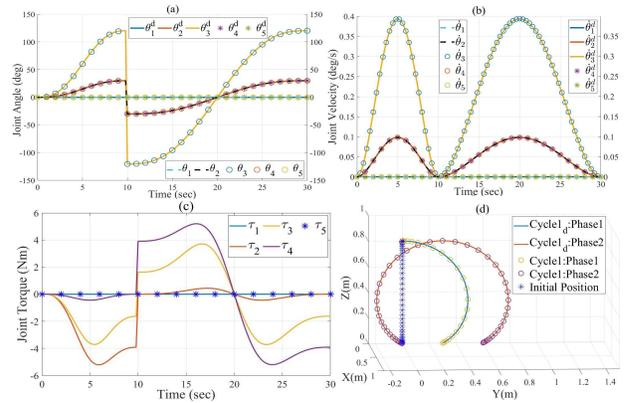
Fig. 4: Outputs: (a) Joint Angles, (b) Joint Velocities, (c) Joint Torques under gravity (d) Trajectory
