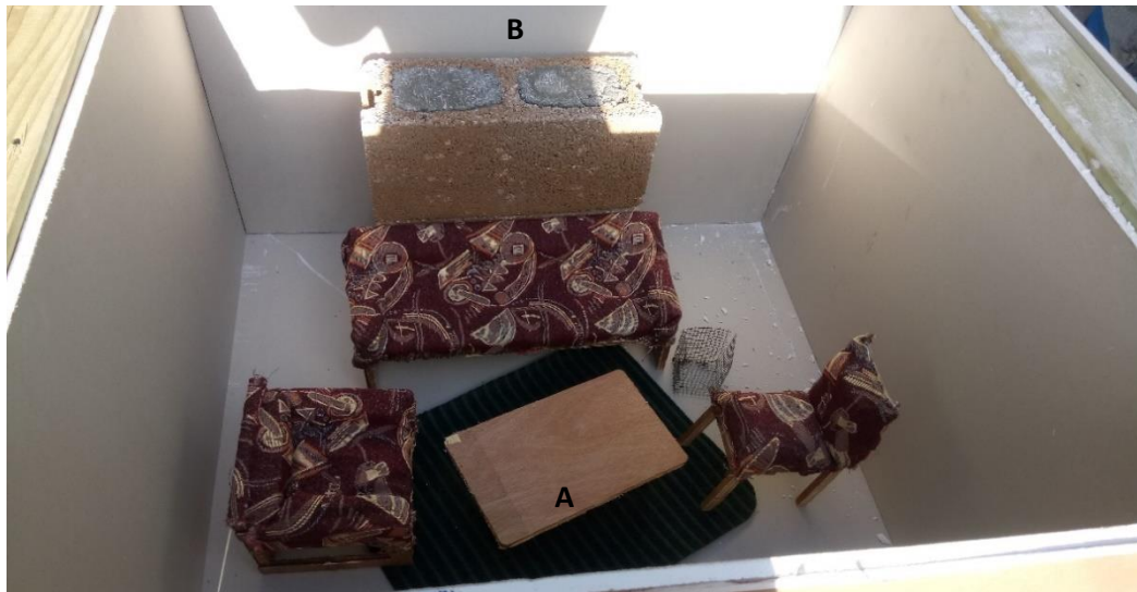
111 Figure 1: Showing a typical fire compartment design used for assessing concrete behaviour at 112 elevated temperatures. A – specifies the front of the compartment; B – specifies the rear of the 113 compartment
