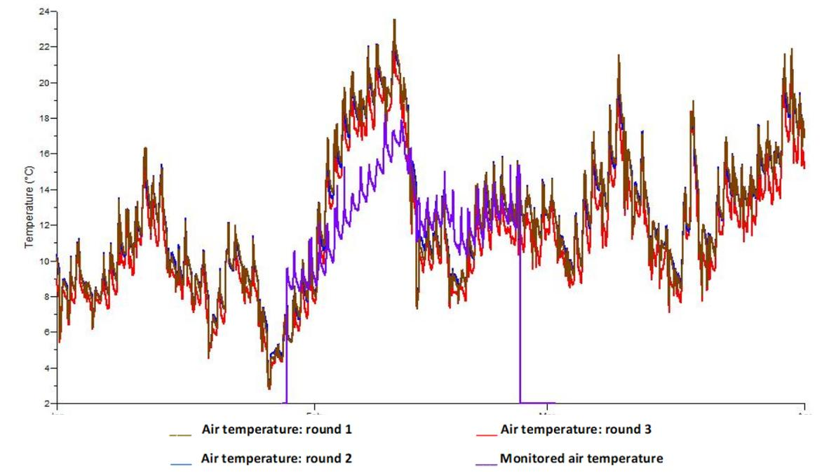
**Figure 6.** Simulation results of the three rounds and the monitored temperature in the living room for the period 12th October-1st November/2017
