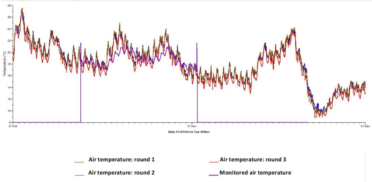
**Figure 5.** Simulation results of the three rounds and the monitored temperature in the living room for the period 12th October-1st November/2017
