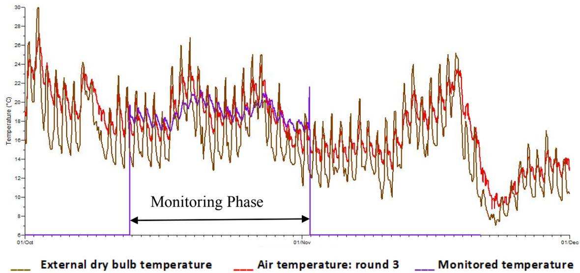
**Figure 7.** Simulation results of the third round in the living room, the monitored temperature and the external temperature for the period 12th October-1st November/2017 (Case 1)
