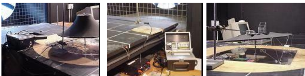
Figure 6. Measurement of the air velocity.
