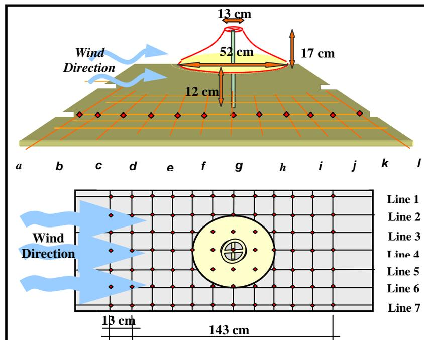
Figure 1. Perspective and plan of the conical membrane structure and the grid of air velocity measuring points
