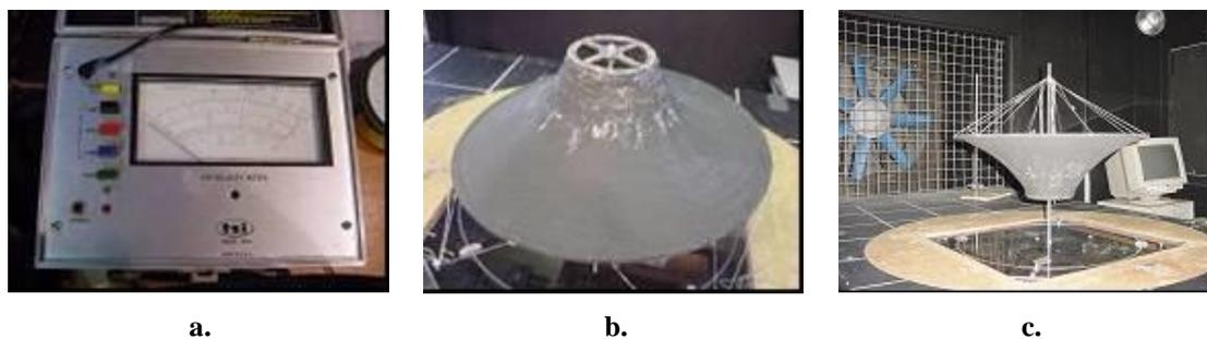
Figure 2. (a) Hot wire anemometer; (b) the conical membrane model; and (c) the model when inclined
