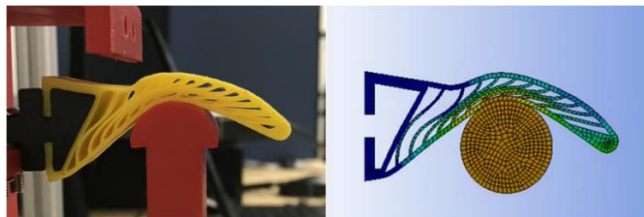
Fig. 2: Visualisation of a deformed Soft FRE finger after layer jamming comparing (a) Experimental test, (b) and corresponding FEA.
