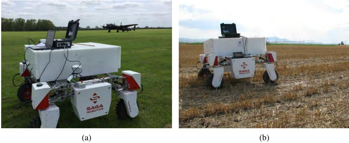
Figure 3: The Thorvald robot equipped with a Cosmic-Ray sensor during data collection at: an airfield at the Lincolnshire Aviation Heritage Centre in East Kirkby, UK (left); a wheat stubble field near Volos, Greece (right).
