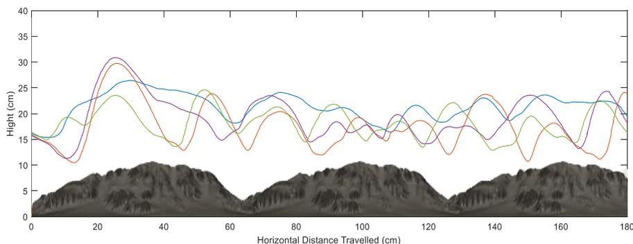
**Fig. 7.** The simulated bee released around the given height in four times. The flight trajectories are shown above the snow mountain terrain in the same graph. Whenever the distance to ground decreases, the angular velocity increases causing the vertical lift goes up, and so does the flight altitude to help it fly over the terrain.
