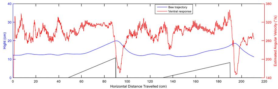
**Fig. 5.** The bee trajectory (blue line), terrain height (black line) and the angular velocity (red line) estimated by the ventral eye are shown in the same graph. A demo video can be found at <https://youtu.be/jaYSuCJGAfc>.
