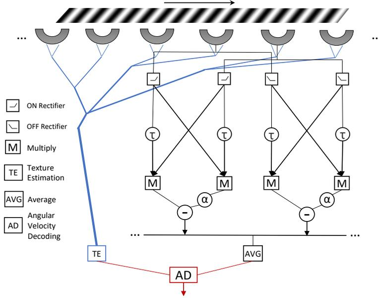
**Fig. 2.** The proposed Angular Velocity Decoding Model. The visual information of the grating movement is received by photoreceptors. The global spatial frequency and image contrast information is estimated by texture estimation part, and the temporal information is processed by motion detectors. Angular velocity decoding layer combines both texture and temporal information to estimate the angular velocity.
