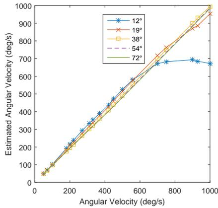
**Fig. 4.** The estimated angular velocity curves from decoding under different angular velocities when tested by moving gratings of different spatial periods ( $12^\circ$ ,  $19^\circ$ ,  $38^\circ$ ,  $54^\circ$  and  $72^\circ$ ).
