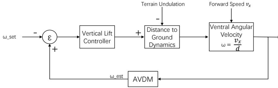
**Fig. 3.** The AVDM-based close loop control terrain following scheme. The vertical lift controller is triggered by the difference  $\varepsilon$  between preset angular velocity  $\omega_{set}$  and the estimated angular velocity  $\omega_{est}$ .
