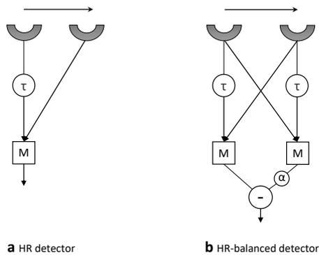
**Fig. 1.** HR detector and HR-balanced detector. (a) HR detector uses the multiplication (M) of the delayed signal from left photoreceptor and the non-delay signal from right to enhance the response of a preferred direction motion [7]. (b) HR-balanced detector can detect both preferred and opposite direction motions [22].
