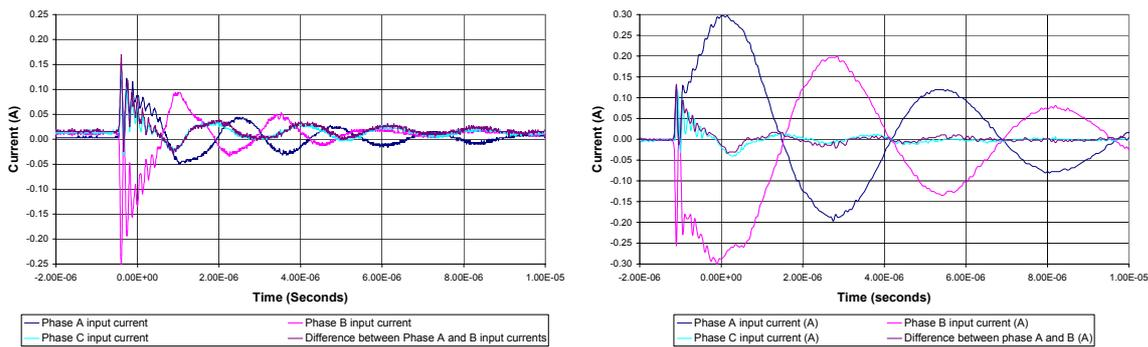
**Figure 14. Current spike occurring on the 3<sup>rd</sup> commutation event (a) without the capacitive load (b) with capacitive load.**
