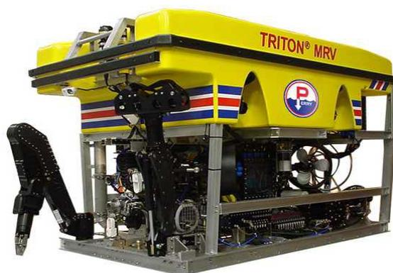
**Figure 1. Deep-Sea (3000m) Remotely Operated Vehicle (ROV).** (Photograph courtesy of Perry Slingsby<sup>1</sup>)
