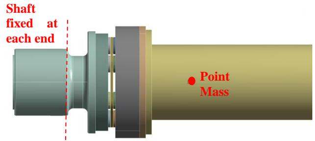
Figure 5. FINITE ELEMENT MODEL OF SHAFT WITH POINT MASS REPLACING SLEEVE
