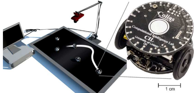
Fig. 1. Artificial pheromone system with 5 Colias robots, LCD screen as the pheromone-enabled ground and an external camera for robot localisation.
