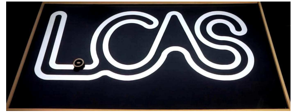
Fig. 5. Localization precision experiment: A snapshot of the experiment with Colias- \Phi robot following a complex path. (LCAS stands for the Lincoln Centre of Autonomous Systems)
